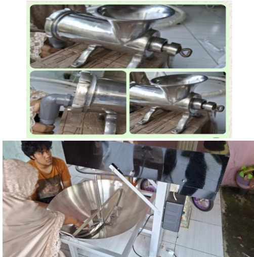
Figure 6. Dodol grinding machine and dodol rolling machine.
